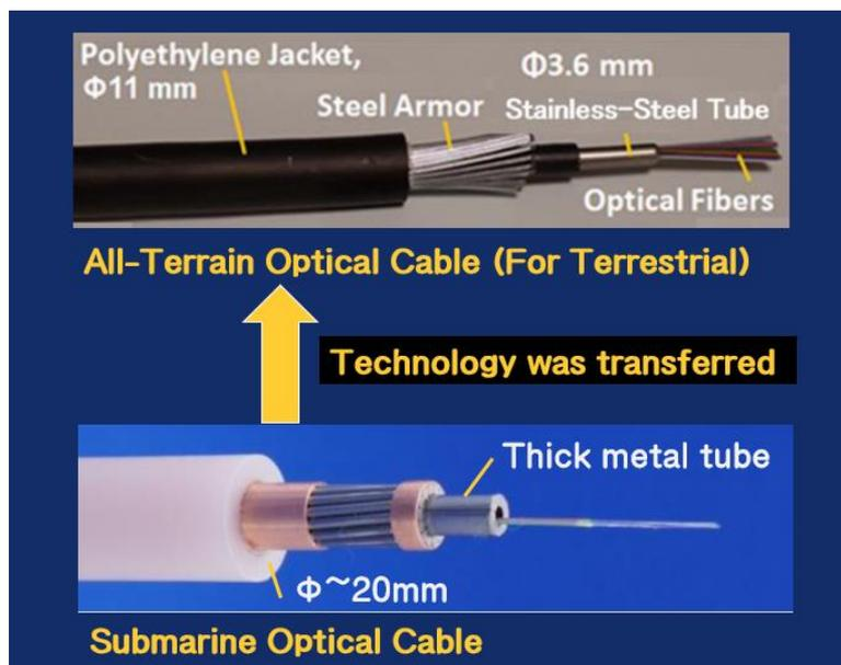
Figure 1 Example of L.110 cable ( upper one) used for the solution BIR
